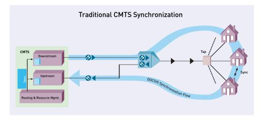
FIG. 1 Cable Modem Termination System Overview
